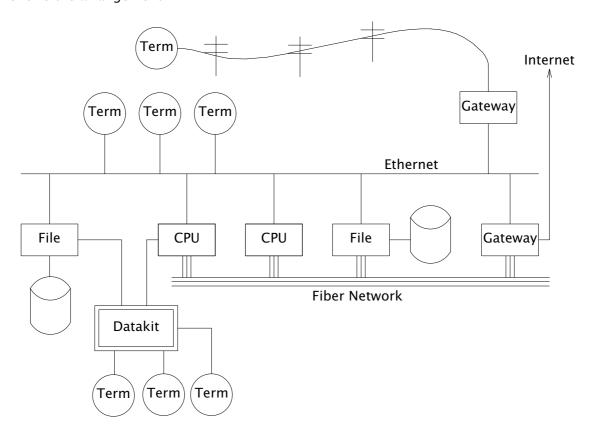
Figure 1. Structure of a large Plan 9 installation. CPU servers and file servers share fast local-area networks, while terminals use slower wider-area networks such as Ethernet, Datakit, or telephone lines to connect to them. Gateway machines, which are just CPU servers connected to multiple networks, allow machines on one network to see another.
